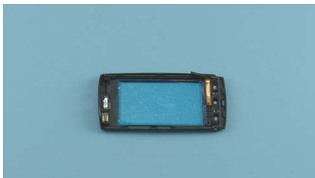
27) Protect the other side of the TOUCH WINDOW with a protective film.
