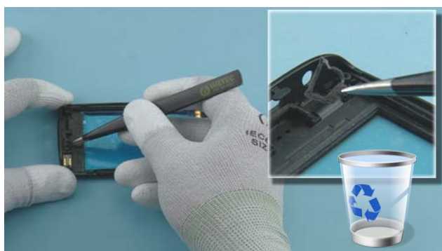
29) Remove also the EARPIECE MESH + GASKET with the tweezers. Do not use it again. Discard it.
