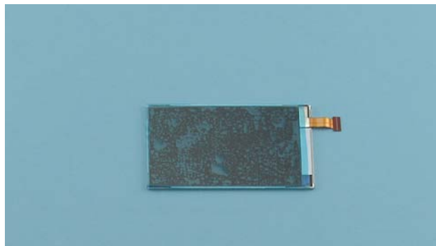
26) Protect the DISPLAY with a protective film.
