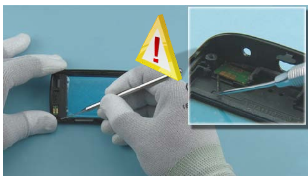
30) Carefully lift up the PROXIMITY SENSOR PWB with the dental tool. Be careful not to damage the PROXIMITY SENSOR PWB.
